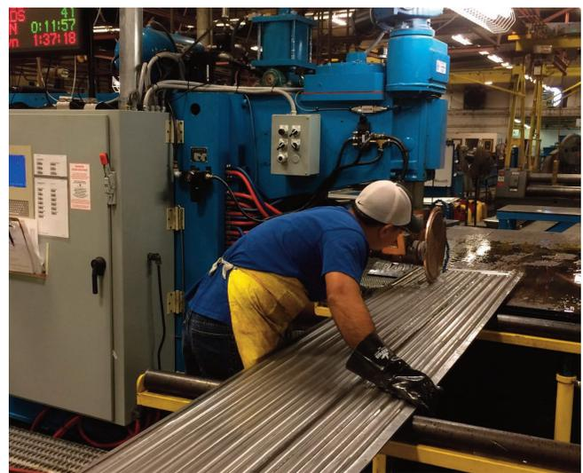
*WeldComputer Adaptive Control producing leak tight seam on heat exchanger.*
