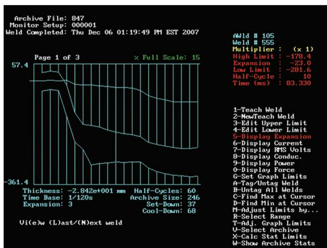
Figure 2. Failed weld 105 showing inadequate set-down response.
