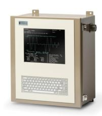
During each weld, Voltage, Current, Conductance, and Power profiles are automatically monitored. Force and Displacement profiles are available options to provide the most comprehensive weld quality monitoring. Any failed check results in an immediate alarm to alert production. The monitor records all data for future proof of weld quality without affecting production throughput.
