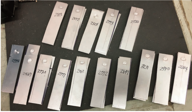
Figure 5. Image of the 15 test welds
