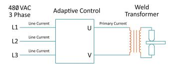
**Example:** A single phase welder that draws 800 amps primary current will draw 656 amps from each power line when connected to a three phase power source with a WeldComputer Control.
