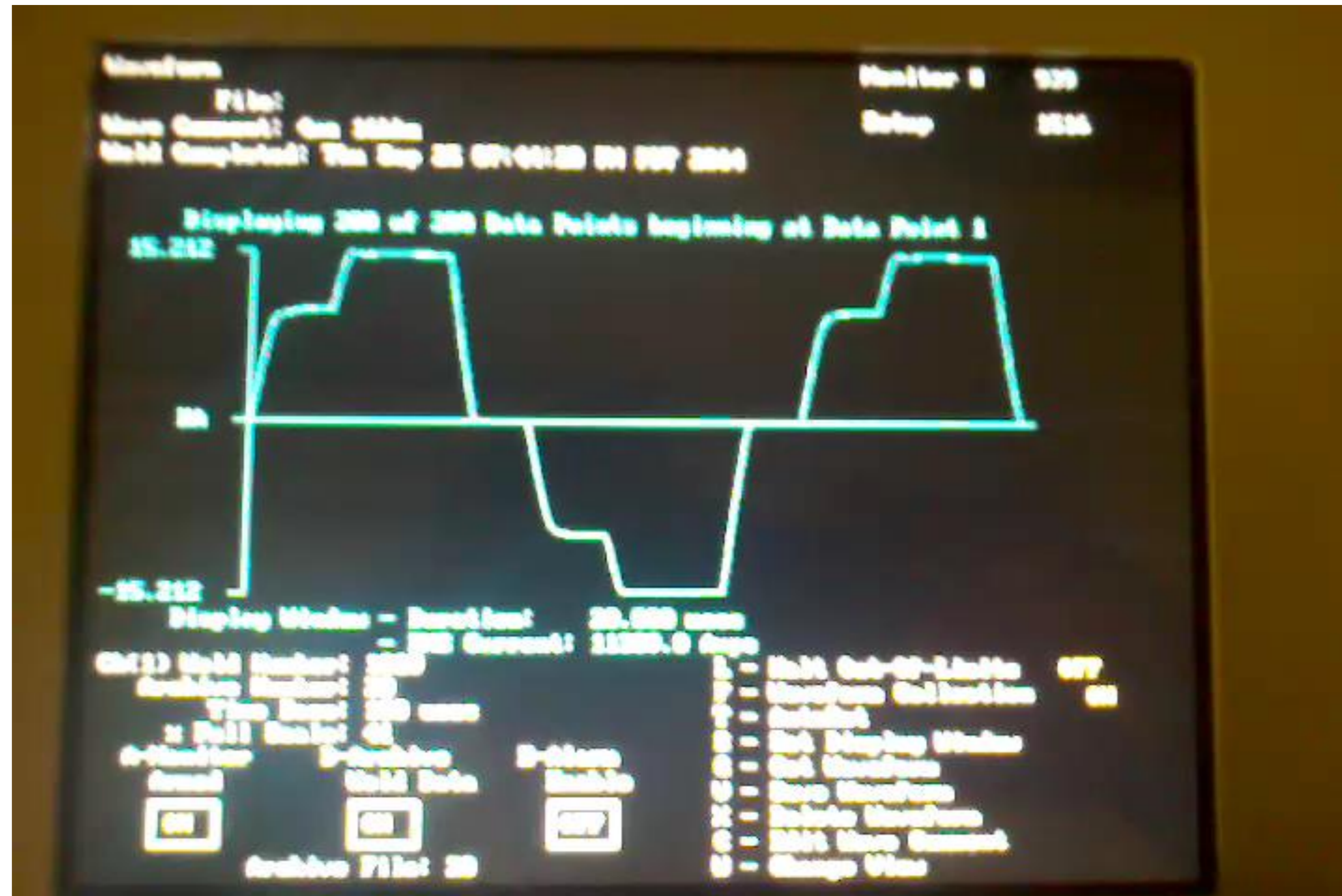
Current trace recorded with WeldView® Monitor
